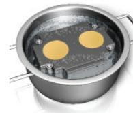
After stone has set, place flask in clean hot water (80°C/175°F) for approx. 5 minutes.
