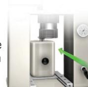
Unscrew the centering disks to release and remove the flask. Place in the Palamat elite for final polymerization.
