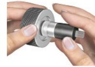
Place the steel injector sleeve over the nozzle.
