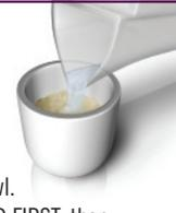
Pour the mix slowly into the prepared cylinder sleeve. DO NOT LET THE MIX RUN DOWN THE INNER WALL OF SLEEVE AND DO NOT CONTAMINATE THE SEALING LIP OF THE SLEEVE.
