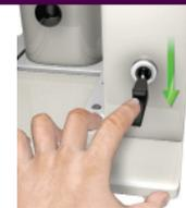
After specified time, flip the air control switch down.
