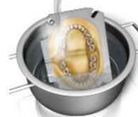
Open flask and remove the remaining wax with clean hot water.
