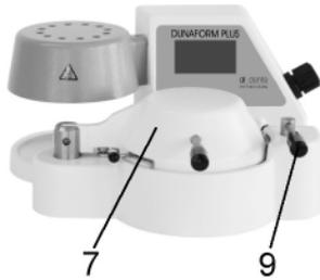
Unlock the pressure chamber (7) by turning the closing device (9) counter-clockwise.
