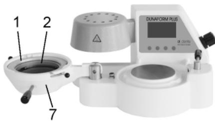
Lift off the pressure chamber (7) and swivel it for 180° all the way. Turn the foil tension ring (1) clockwise and take it off.
