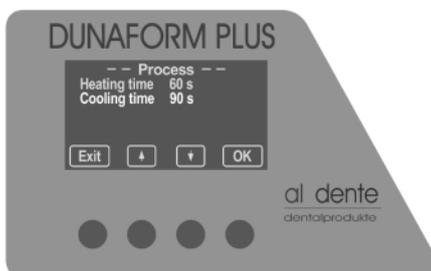
Display (4) shows: Process, Heating time 60 s, cooling time
