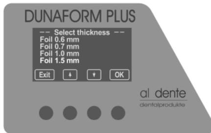
Display (4) shows: Select thickness, Foil 0.6 mm, Foil 0.7 mm, Foil 1.0 mm, Foil 1.5 mm.
