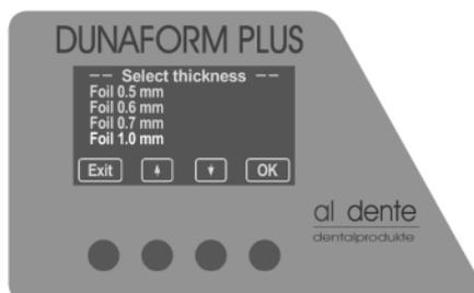
Display (4) indicates: Select thickness, Foil 0.5 mm, Foil 0.6 mm, Foil 0.7 mm, Foil 1.0mm.
