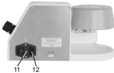
The fuses are situated in the female connector installed (12).
