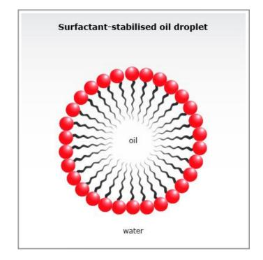
In the development of RESINAWAY®, we use the principal of Micelle development to produce chemistry with "Critical Micelle Concentration", ending up with enough Micelles to create a stable emulsion of residual 3D resin that will wash cleanly off 3D printed parts.
