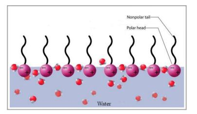
When you have enough surfactant in solution, it will begin to move downwards into the water phase to create micelles – a fundamental component of any surfactant-based product. Micelles form little balls in oil at hydrophobic substances with the tails all facing inwards, trapping the once surface oil in between, to form into stable droplets as is the case in lotions when you have enough micelles in the solution.
