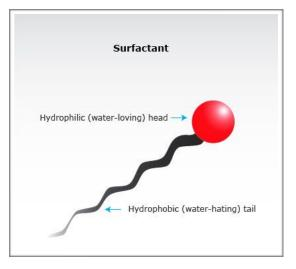
The surfactant component illustrated above combine to form a "Micelle" where a ball cluster forms with the tails facing inwards say into a droplet of hydrophobic oil like substance and the Hydrophilic water-loving Heads covering the outer surface of the oil-like droplet thus forming a contact with the surrounding water. When all the oil is taken up as above, the whole mass is then water miscible – oil now soluble in water.
