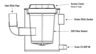
**NOTE:** Internal pipe configurations vary according to tank type capacity and/or customer requirements. The above drawing is indicative only. The installer must comply with local regulations when connecting a trade waste tank.
