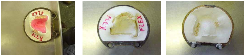
Fig. 2 Wax up investment in flask. boil out and apply separator.
