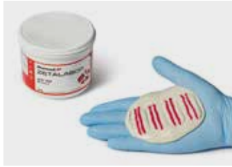
3. Measuring and mixing Zetalabor (4 measures)
