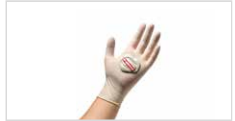
3. For each measure, spread two strips of Zhermack Indurent Gel catalyst the same length as the measure, i.e. about 4 cm
